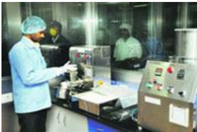
The neutral spheres development using extruder and spheroniser
