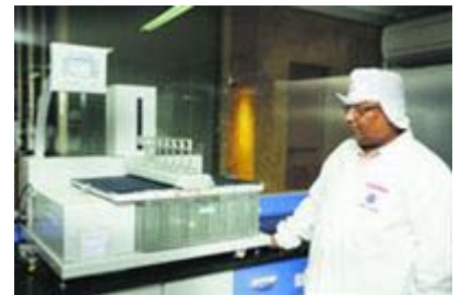
Critical observations on dissolution profile of ER tablets on USP Type III apparatus
